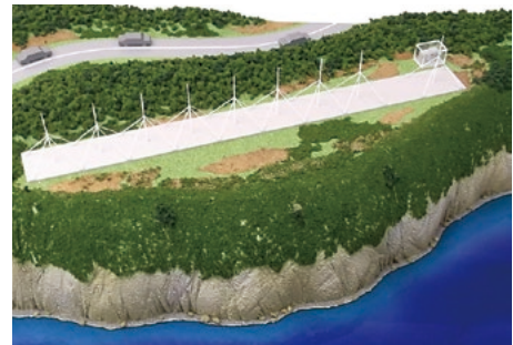
Fig. 1 Image of ocean surface radar transmission and receiving antennas
