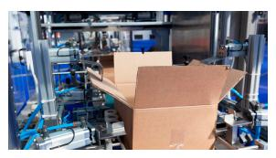
Simple synchronous operations including horizontal, vertical, and rotational movements are possible with a start signal to all axes via cyclic transmission. This function can be used to easily build a multi-axis system for packaging, etc.
