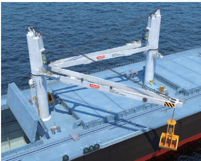
Electric deck crane (P.9)
