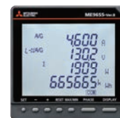
Electronic multi-measuring instruments ME96SS series
