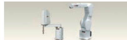
Robots: SCARA, Articulated arm
