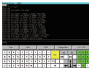
[Editing Motion programs] G-code programs from a Motion controller are displayed as a list and edited on GOT.
