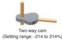
Reciprocating operation with a constant cam strokes range
