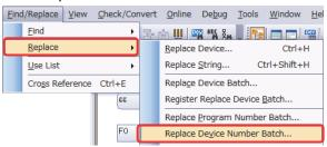
2) Select "Replacing with specified K/F/G program range" tab. Enter the device numbers in [(a) Replace From:] [To:], and [(b) Replace With:]. Click [Check >> Execute].
