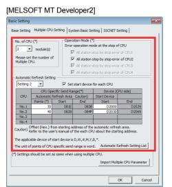
(b) Multiple CPU setting of RnCPU and RnMTCPU
