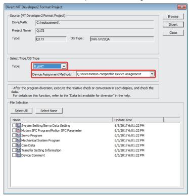
5) Check the box of the data to be diverted in the "File Selection". Click "Divert". When projects for Q17nCPUN(-T) are diverted as those for RnMTCPU, remove the check of the "Transfer Setting Information" box since the "Transfer Setting Information" cannot be diverted.
