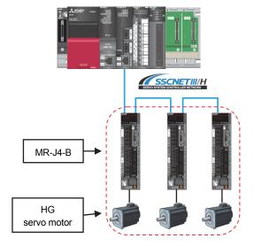
(Note): When replacing all the servo amplifiers with MR-J4-B, the operation mode can be switched from "J3 compatibility mode" to "J4 mode". The servo system network is also changed from SSCNETIII to SSCNETIII/H.
