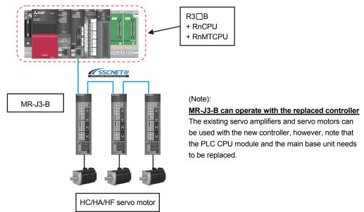
(2) When the MR-J3-B servo amplifier has malfunctioned. Replace only the servo amplifier.
