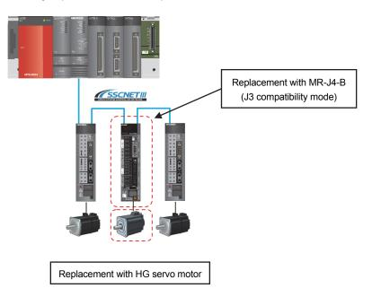
(3) When the HC/HA/HF servo motor has malfunctioned Simultaneously replace the servo amplifier and the malfunctioned servo motor.
