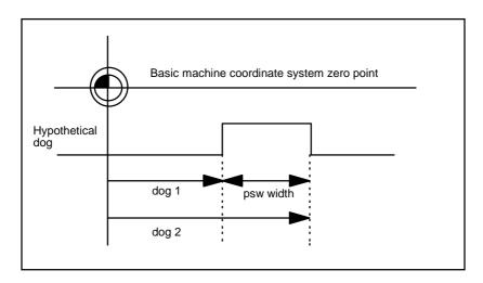
Set the coordinate position of the position switch using the basic machine coordinate system as a reference.
