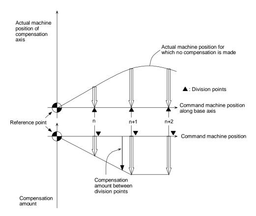
Fig. 2 Relationship between base and compensation axes
