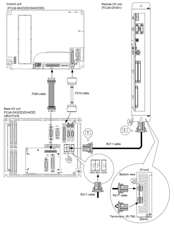
(Note) When not expanding the remote I/O units, connect the terminator (R-TM) to RIO2.
