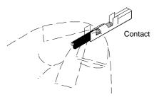
4. Firmly press down the other side of the wire barrel.(Press firmly enough that the wire will not come out when pulled lightly.)
