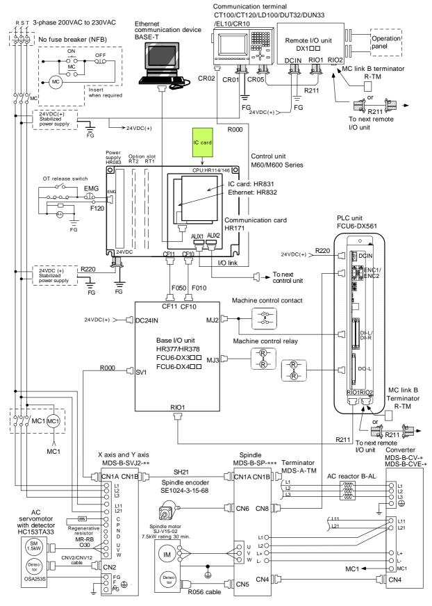
(Note) This drawing is an example of the general connection for the M60/M600 Series. The actual connection will differ according to the specifications.
