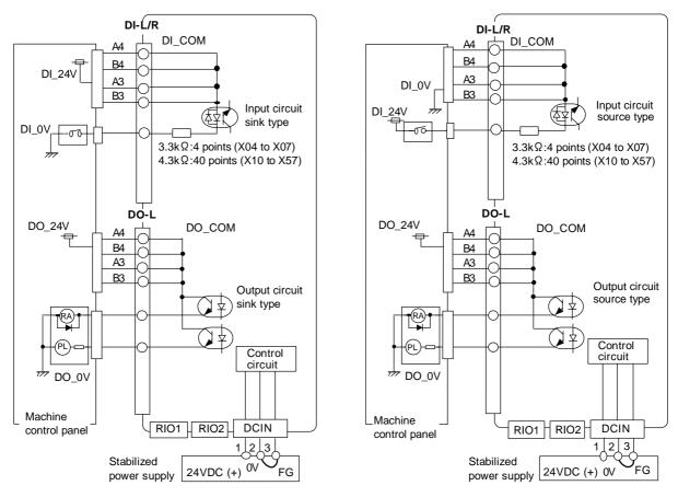
The input circuit can be switched to a sink type or source type with the connections. The output circuit is fixed to the source type.
