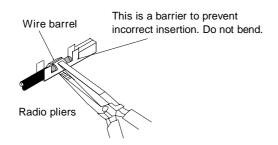
5. Firmly press down the sheath retainer in the same manner as the wire barrel.
