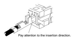
2. Insert the wire into the contact. Hold the sheath retainer.
