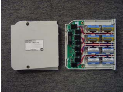
Example of incorporated batteries (Photo: 8 batteries incorporated)
