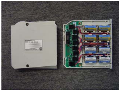
Example of incorporated batteries (Photo: 8 batteries incorporated)
