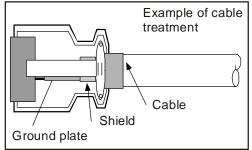
Fold the wire material shield over the sheath, and wrap copper foil tape over it. Then clamp it with the connector's GND plate.
