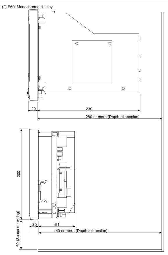
(Note 1) When the display unit is FCU6-DUT11 (LCD), apply the depth dimension of the figure above. (Note 2) Depth dimension includes the space for wiring. Refer to "3.4 Installation" also.
