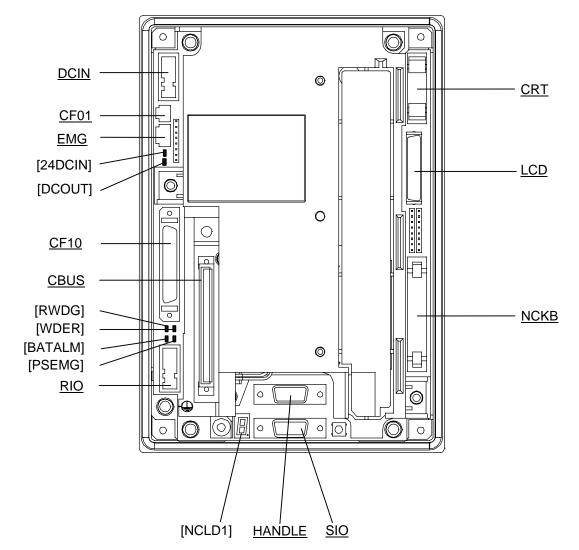
(Note) The underlined names are names of connectors.
