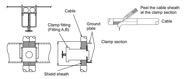
As for the outline drawings of ground plate and clamp fitting, refer to Appendix 1.9 Outline drawing of ground plate and clamp fitting.
