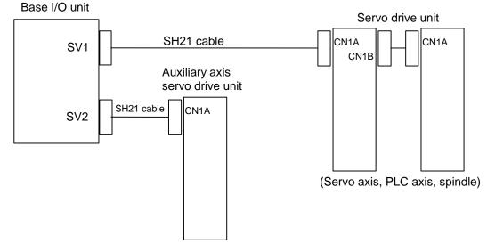
Connect the terminal resistor (FCUA-A-TM) to the terminal end of the servo drive unit. <Related items>
