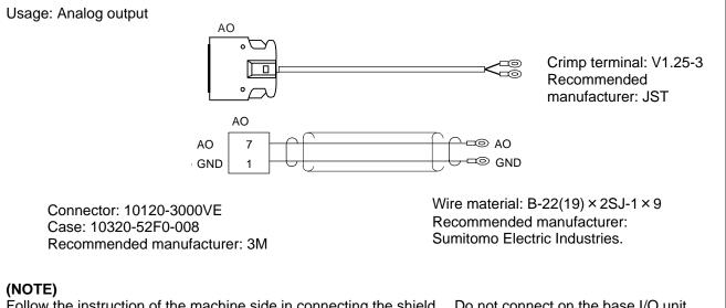
Follow the instruction of the machine side in connecting the shield. Do not connect on the base I/O unit side.
