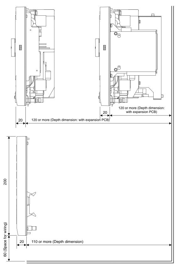
(Note 1) Depth dimension includes the space for wiring. Refer to "3.4 Installation" also.
