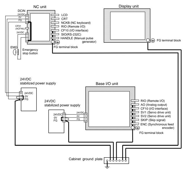
(Note 1) The means that the metal case of the connector is connected to the FG terminal block by the FG pattern on the board.
