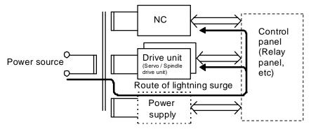
Figure 1. Damage route by lightning surge
