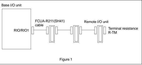
Connect the terminal resistor to the terminal end of the remote I/O unit connected to the connector RIO. Model name of the terminal resistor: FCUA-R-TM
