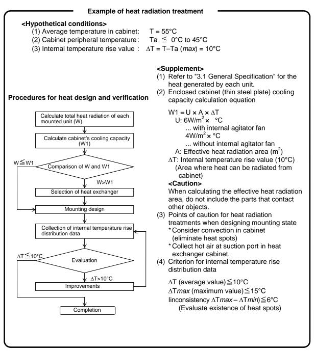
For heat radiation value of each unit, refer to "3.1 General Specification". If heat won't escape from the upper part of the NC unit, equip an agitator fan.
