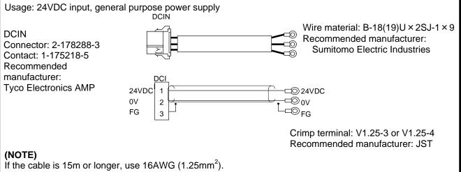
Select the crimp terminal suitable for the terminal block and external power supply you use.
