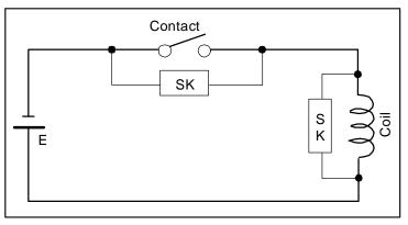
The CR compound element is effective to remove noises caused by electromagnetic induction.
