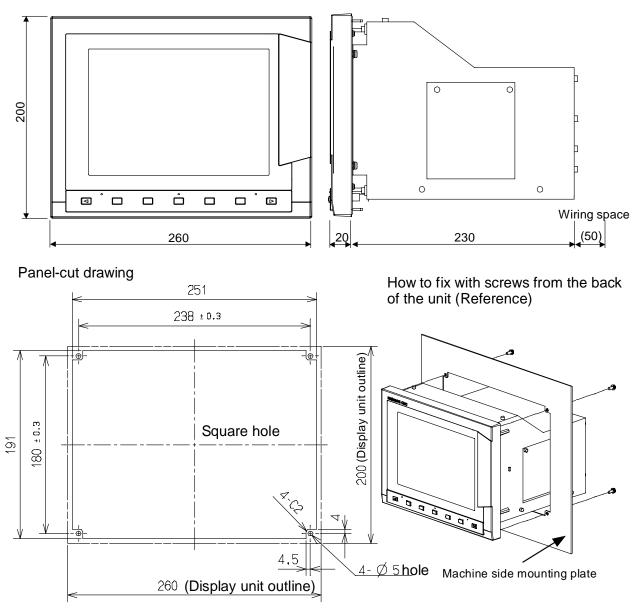
(2) In the case of FCU6-DUE071-1 (Fix with screws from the front of the unit)
