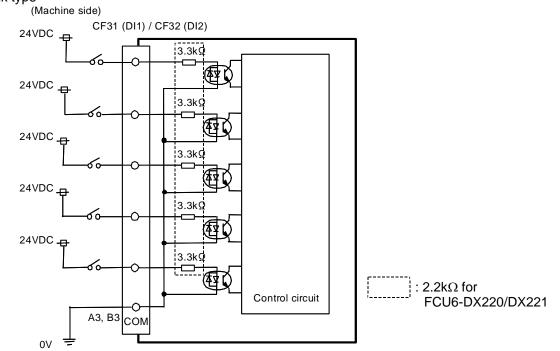
(2) Conditions for input The input signals must be used within the following condition ranges. Sink type
