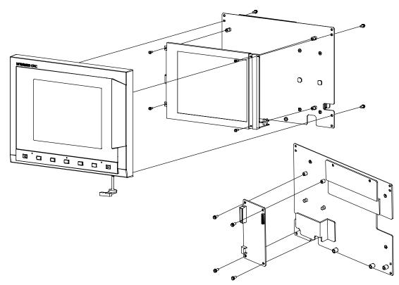
In case of replacing the back light power supply PCB (HR721) at the back of the display unit, turn the electric cabinet power OFF before the replacement.
