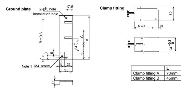
(Note 1) Screw hole for wiring to ground plate of cabinet.
