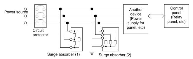
Figure 2. Lightning surge measurement in the case of three-phase power supply
