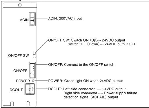
(Note) For usual turning ON/OFF, use the ON/OFF switch of the operation board.
