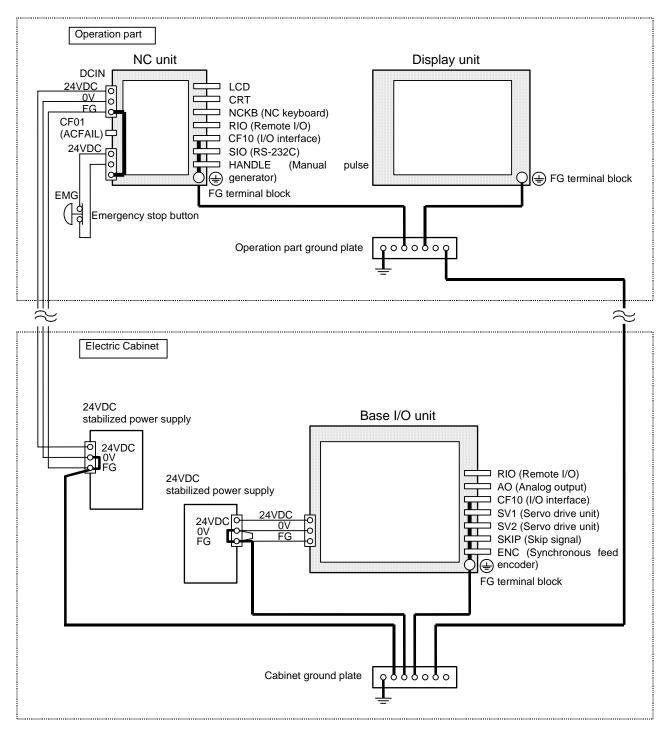
(Note 1) means that the metal case of the connector is connected to the FG terminal block by the FG pattern on the board.
