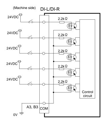
(2) Input conditions The input signals must be used within the following condition ranges. Sink type
