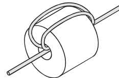
Lead through three times (three turns)
