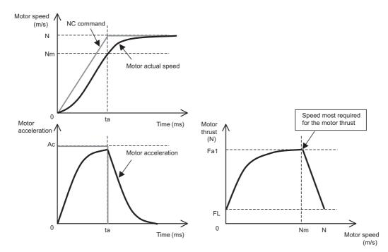
Fig.1 Speed, acceleration and thrust characteristics when using the NC command linear acceleration/deceleration pattern + servo standard position control
