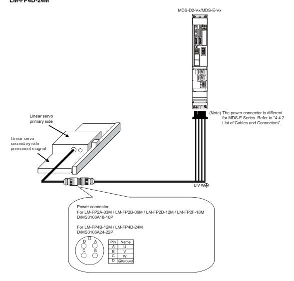
(2) < When the power supply output of the servo drive unit is a terminal type > Connecting the following linear motors LM-FP4F-36M LM-FP4H-48M LM-FP5H-60M
