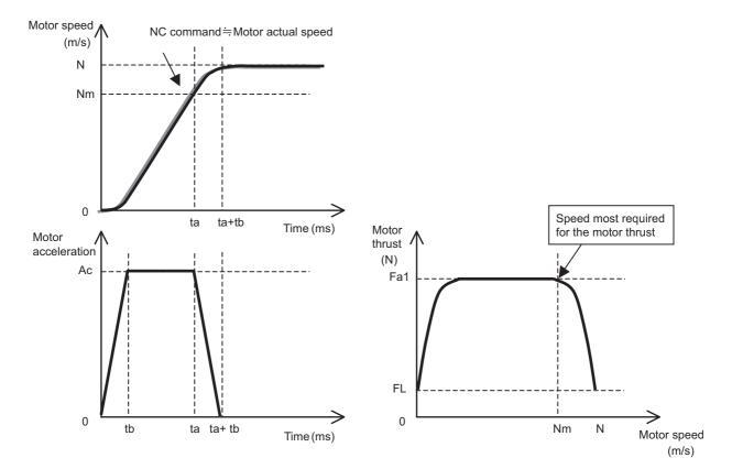
Fig 3. Speed, acceleration and thrust characteristic when using the NC command soft acceleration/deceleration pattern + feed forward control
