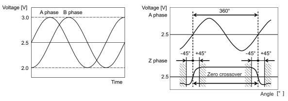
A/B phase output signal waveform during forward run
