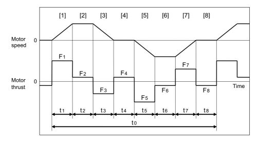
Fig. 5-1Continuous operation pattern
