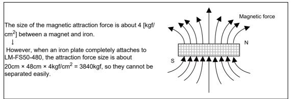
Especially if two secondary sides are placed close to each other, it is highly dangerous as the magnetic attraction force will be greatly strong. For the secondary side, take the sufficient safety measure.
