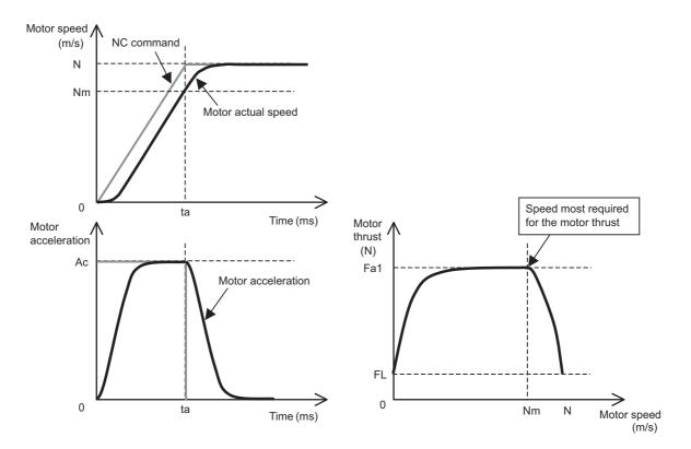
Fig.2 Speed, acceleration and thrust characteristics when using the NC command linear acceleration/deceleration pattern + servo SHG control
