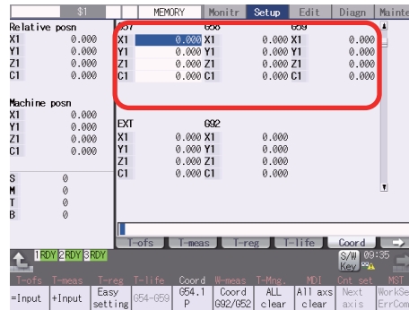
Changed to the next workpiece coordinate system offset (G57-G59) page.
