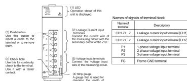
Check the stripping length using the strip gauge of this module
