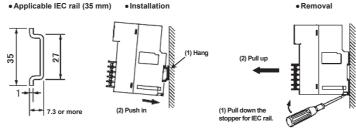
To install IEC rails, secure them using M4 or M5 screws at intervals of 25 to 100 mm. When installing IEC rails in series, secure each end of the IEC rails with sideslip prevention clamps When reinstalling the product onto an IEC rail after removal, install it with the IEC rail stopper pushed in
