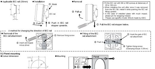
Attach the display unit from front side of panel, and tighten the screw from
