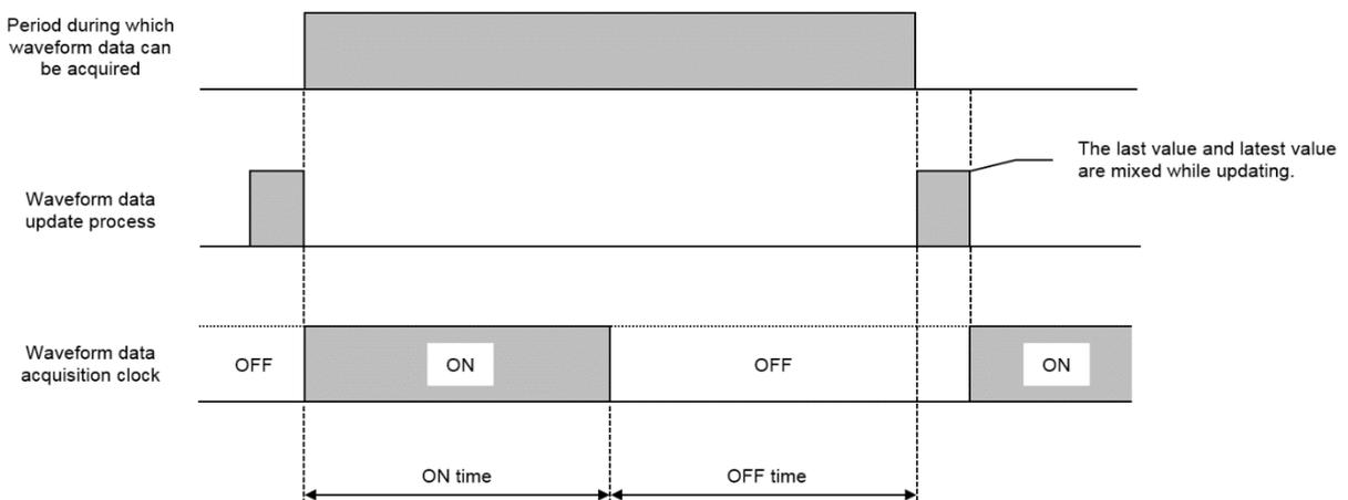
(7) Measured harmonics data acquisition clock (Xn7)
