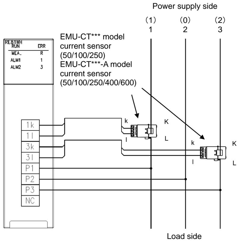
Figure 6.3.3-5 In the case of Single-phase 3-wire
