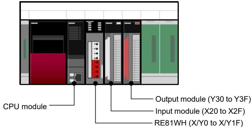
Figure 7.2.1-1 Sample system configuration using a sample program
