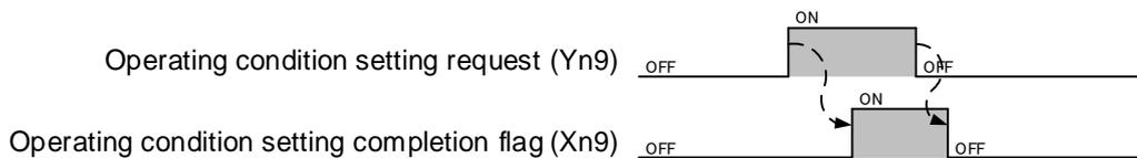
Figure 3.4.4-1 Time chart of alarm monitoring setting
