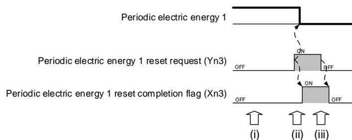
Figure 3.4.2-2 How to reset the periodic electric energy 1
