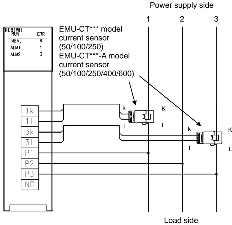
Figure 6.3.3-3 In the case of Three-phase 3-wire system
