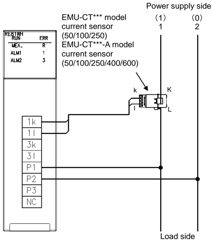
Figure 6.3.3-4 In the case of Single-phase 2-wire system
