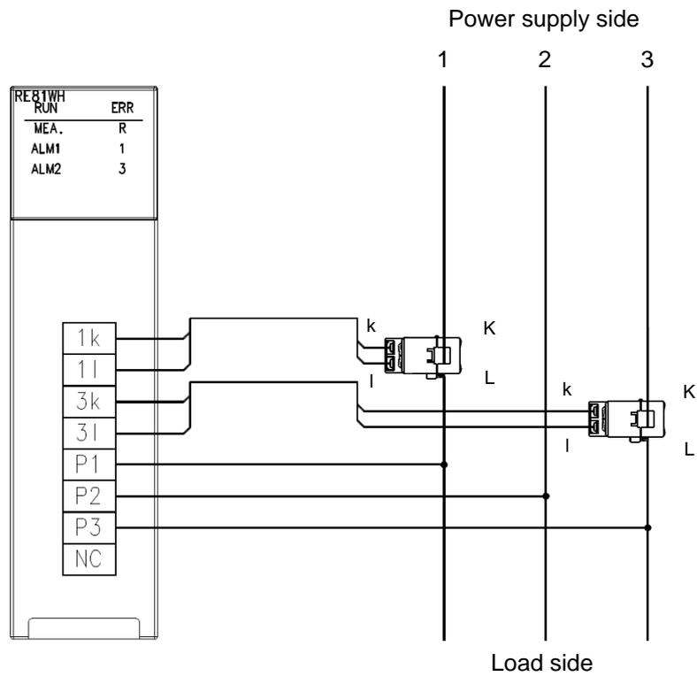
Figure 7.2.3-1 Example of wiring using a sample program
