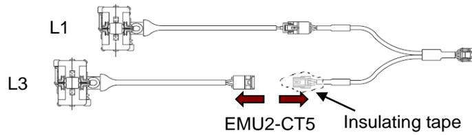
■ Extending the cable of 5 A current sensor
