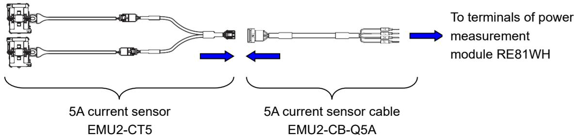
Follow the procedure below to attach the cable to the target circuit.
