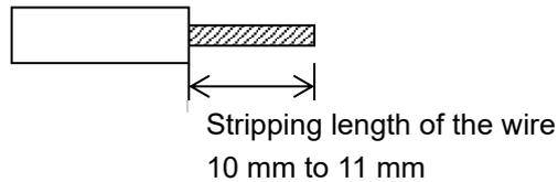
(4) When stranded wire is used, a bar terminal must be used.
