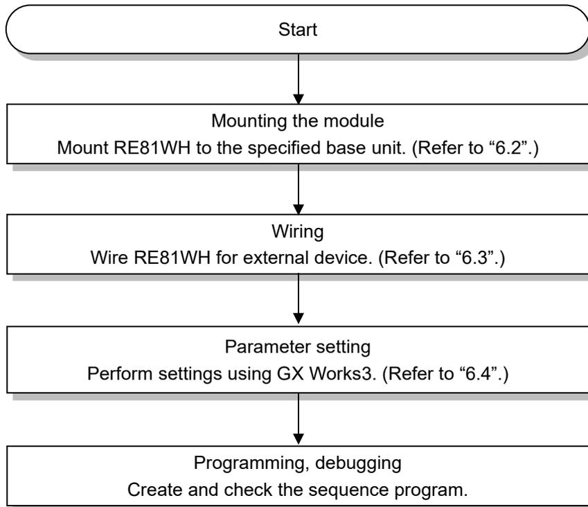
Figure 6.1-1 Procedure for operation
