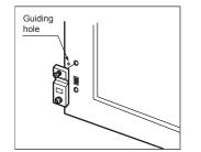
(2) When the USB interface is not used, also tighten the lower fixing screw of the USB environmental protection cover within the specified torque range (0.36 to 0.48 N•m). (IP67f compliant)
