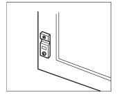
(3) When the USB interface is used, remove the lower fixing screw of the USB environmental protection cover, and connect the USB cable. (IP67f incompliant)
