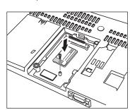
(4) Fasten the multi-color display board by tightening its fixing screw with tightening torque 0.25 to 0.35 N·m.
