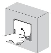
Peel the release paper off the back of the new protective sheet. 2) With the protective film left on the sheet surface, attach the sheet on the GOT so that the USB environmental protection cover hole is just on the USB environmental protection cover of the GOT.
