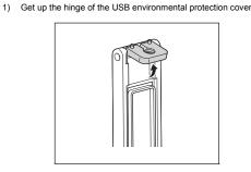
Put the provided fixing screw through the hinge hole, and then fit the screw in the cover installation hole on the GOT.
