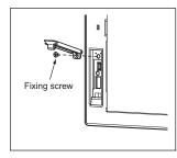
3) Tighten the screw with a torque of 0.36 to 0.48N•m Fitting the hinge projections in the GOT guiding holes makes the cover installation work easier.
