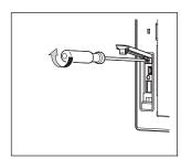
4) When the USB interface is not used, fix the cover by pushing the △ mark on the latch firmly.
