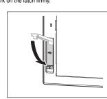
When the USB interface is used, unfix the latch to open the cover, and then connect the USB cable.
