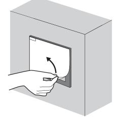
Peel the release paper off the back of the new protective sheet. 2) With the protective film left on the sheet surface, attach the sheet so that the POWER LED hole is just on the POWER LED of the GOT.
