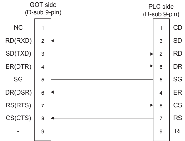
RS232 connection diagram 4)
