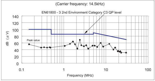
(Note) Ferrite core is wrapped two turns around the parameter unit connection cable.
