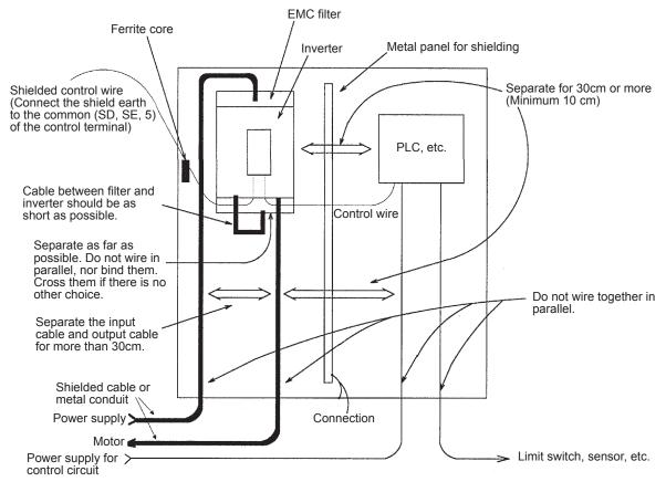
(6) Inserting the line noise filter FR-BLF or FR-BSF01, which is described in Chapter 4, into the input or output side of the inverter improves the interference reduction effect.
