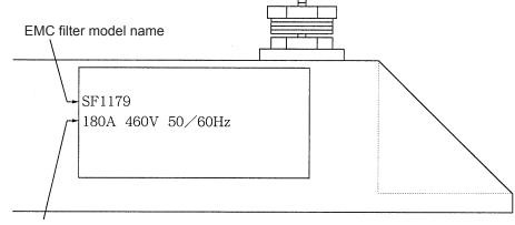
Rated current, rated voltage, power supply frequency
