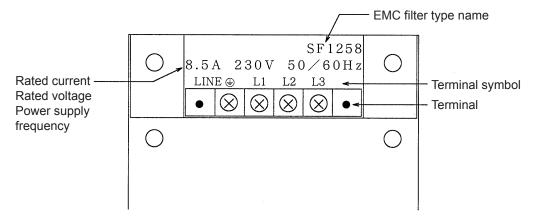
Example of the rating plate on the side or the front of the EMC filter
