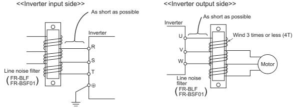
(7) Ensure to ground (earth) at the motor side.
