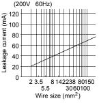
Fig. 2-3 Leakage current example of three-phase induction motor during the commercial power supply operation
