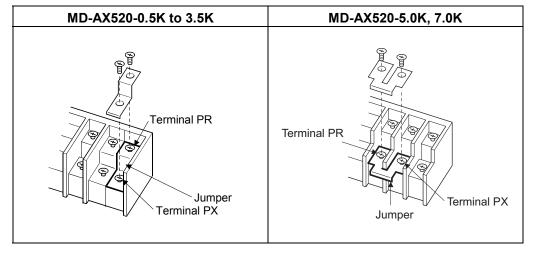
2) Connect the brake resistor to the terminals P/+, PR.
