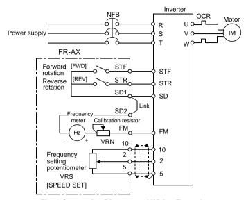
Fig. 4 Connection Diagram and Wiring Example
