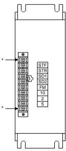
Fig. 5 Terminal Layout Diagram
