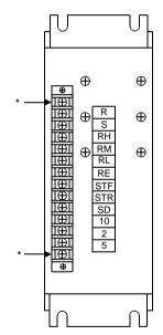
Fig. 5 Terminal Layout Diagram
