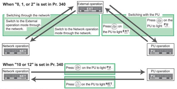
For the switching method with the external terminal, refer to *the Instruction Manual of the inverter*. Refer to *page 69* for a switching method through the network.
