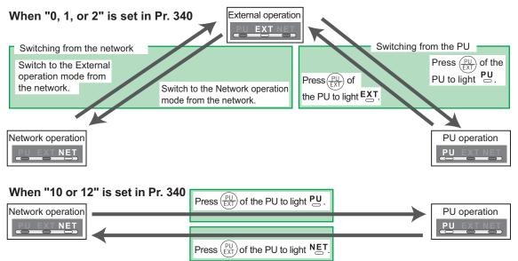
For the switching method from the external terminal, refer to *the Inverter Manual*. Refer to *page 58* and *81* for a switching method from the network.
