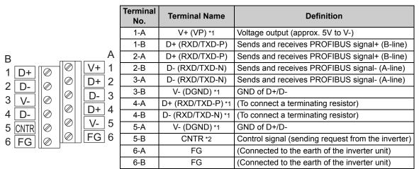
\*1 Use this when connecting a terminating resistor.
