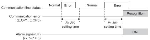
When a communication line error occurs and lasts longer than the time set in *Pr*: 500, it is recognized as a communication error.
