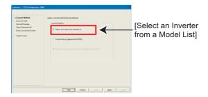
3) Set the information of the source inverter in "Model Setting". Fill in the each item of the source inverter. Click after setting.
