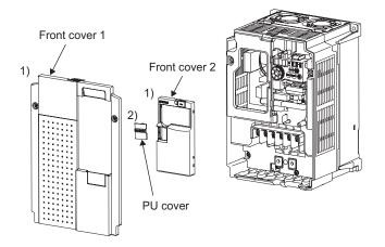
Because the voltage class is stated on the PU cover, replace a PU cover of a plug-in option front cover with the removed PU cover from the inverter.
