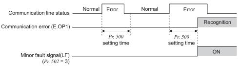
If the communication line error still persists after the time set in *Pr. 500* has elapsed, it is recognized as a communication error.
