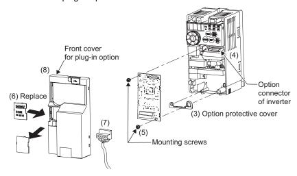
When the option protective cover is not installed, the protective structure (JEM1030) changes to open type (IP00).
