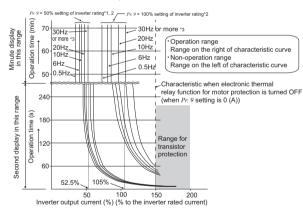
This function detects the overload (overheat) of the motor, stops the operation of the inverter's output transistor, and stops the output.
