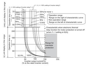
This function detects the overload (overheat) of the motor, stops the operation of the inverter's output transistor, and stops the output. (The operation characteristic is shown on the
