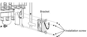
(3) Reconnect the fan connector, and then place the connector case from the above.
