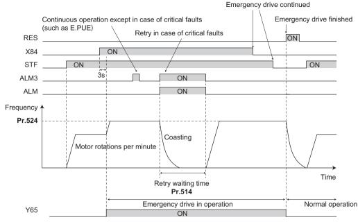
The following diagram shows the operation of switching over to the commercial power supply operation during emergency drive operation by using the CS signal (when the electronic bypass during emergency drive operation is enabled) (in the commercial mode or in the fixed frequency mode (**Pr.523** = "411")).
