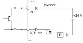
External signal input using transistor (sink logic)
