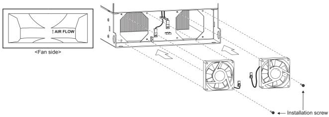
(2) Route the fan lead through the clamp, and then reconnect the fan connectors.
