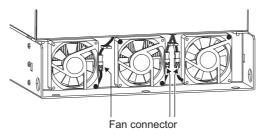
(3) Remove the installation screws, and then remove the fan.
