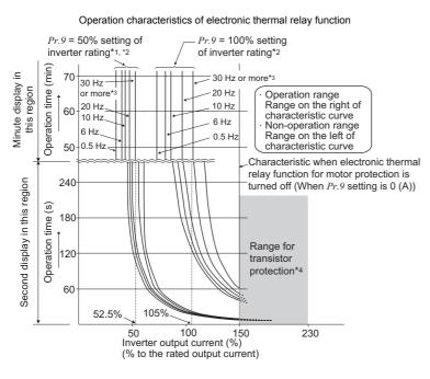
This function detects the overload (overheat) of the motor, stops the operation of the inverter's output transistor, and stops the output. (The operation characteristic is shown on the left.)
