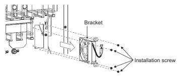
(4) Remove the installation screws, and then remove the fan.
