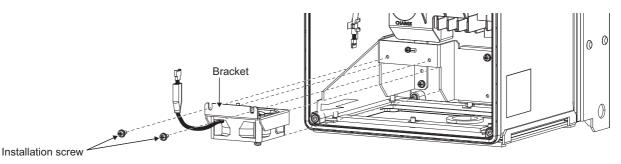
(4) Remove the installation screws, and then remove the fan.
