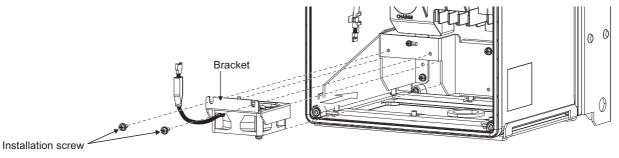
(3) Reconnect the fan connector, and then place the connector case from the above.
