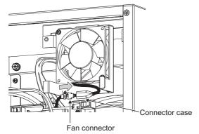
(3) Remove the installation screws, and then remove the bracket.
