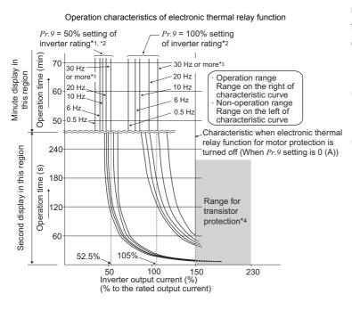
This function detects the overload of the motor, stops the operation of the inverter's output transistor, and stops the output. (The operation characteristic is shown on the left.)
