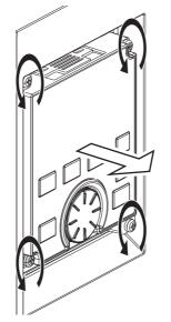
• To reinstall the operation panel, align its connector on the back with the PU connector of the inverter, and insert the operation panel. After confirming that the operation panel is fit securely, tighten the screws in the diagonal order. (Tightening torque: 0.39 to 0.49 N·m)
