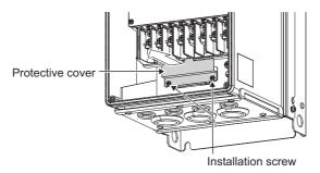
(3) Move the fan connector case, and then remove the fan connector.
