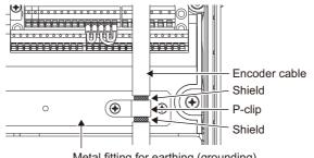
Metal fitting for earthing (grounding)
