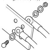
• When wiring the main circuit conductor (terminals R/L1, S/L2, T/L3) of the converter unit (FR-CC2), use the bolts (nuts) for main circuit wiring, which are provided on the front side of the conductor.
