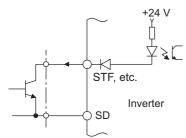
External signal input using transistor (sink logic)
