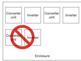
Arrangement of multiple inverters and converter units
