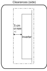
\*1 For replacing the cooling fan, 30 cm or more of space is necessary in front of the inverter. Refer to page 76 for fan replacement.
