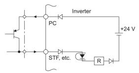
External signal input using transistor (source logic)
