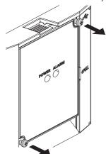
Push the upper part of the accessory cover and pull the accessory cover to remove.
