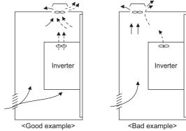
Arrangement of the ventilation fan and inverter
