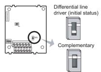
Terminating resistor selection switch (SW1)
