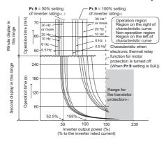
This function detects the overload (overheat) of the motor and trips the inverter by stopping the operation of the transistor at the inverter output side. (The operation characteristic is shown on the left.)
