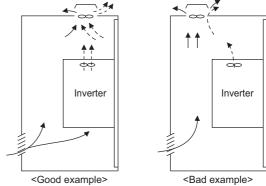
Arrangement of the ventilation fan and inverter
