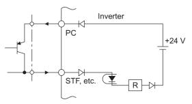
External signal input using transistor (source logic)
