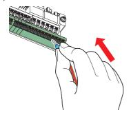
When using single wire or stranded wires without a crimp terminal, push the open/close button all the way down with a flathead screwdriver, and insert the wire.
