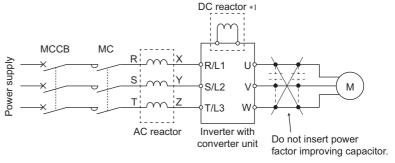
\*1 The converter unit (FR-CC2-C) is equipped with the DC reactor.
