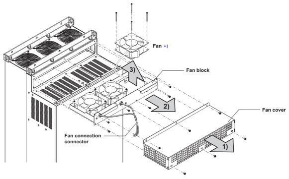
\*1 The number of cooling fans differs according to the inverter capacity.
