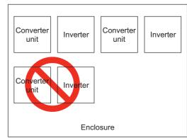
Arrangement of multiple inverters and converter units
