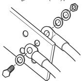
• When wiring the main circuit conductor (terminals R/L1, S/L2, T/L3) of the converter unit (FR-CC2-C), use the bolts (nuts) for main circuit wiring, which are provided on the front side of the conductor.
