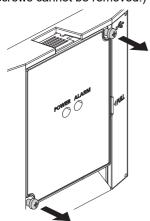
Push the upper part of the accessory cover and pull the accessory cover to remove.
