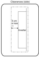
\*1 For replacing the cooling fan, 30 cm or more of space is necessary in front of the inverter. Refer to page 70 for fan replacement.
