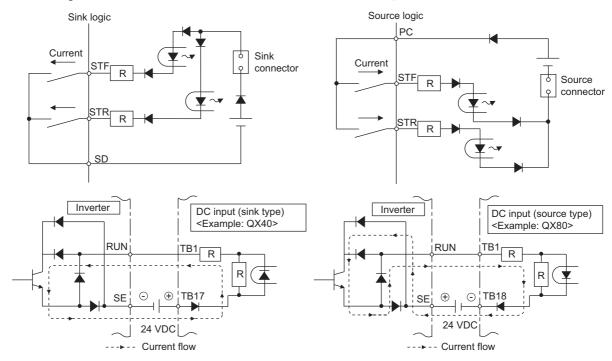
· When using an external power supply for transistor output
