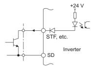
External signal input using transistor (sink logic)
