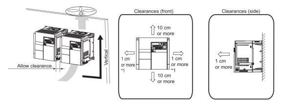
\*1 When using the inverters at the surrounding air temperature of 40°C or less, the inverters can be installed closely attached (0 cm clearance).
