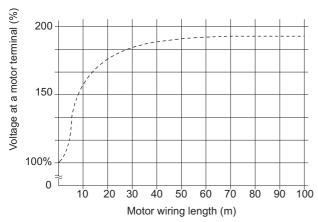
Surge voltage at a motor terminal by motor wiring length (reference)
