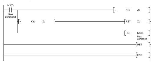
To the next command. Z0 = 0:Load current (I11) Z0 = 10:Electric energyZ0 = 20:Alarm/fault cause
