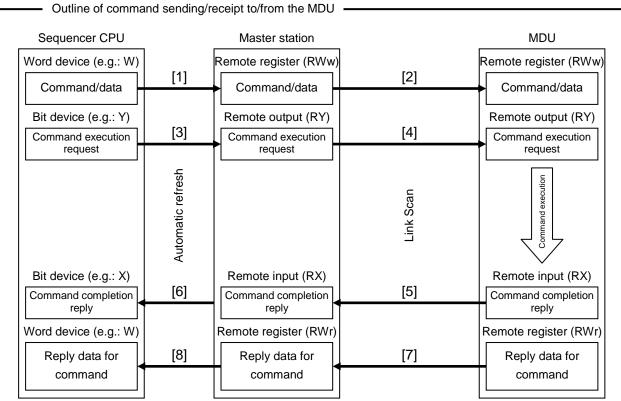
[1] By the automatic refresh, commands and the associated data stored in the word device of the sequencer CPU are stored in the remote register (RWw) of the master station.
