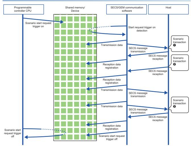
In the course of transaction operations within a scenario, the software refers to (for sending) or writes data to (for receiving) the related register without controlling the trigger relay.
