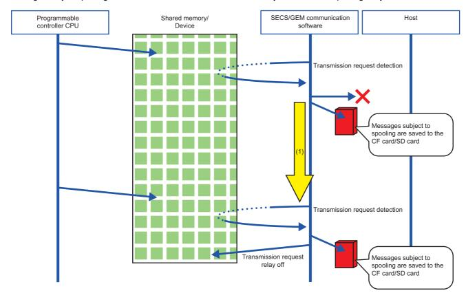
(1) The spooling relay is ON.
