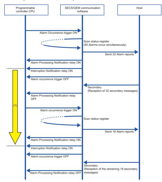
(1) Locked by the ladder program so that alarm recovery processing is not carried out until all alarm report sending is complete
