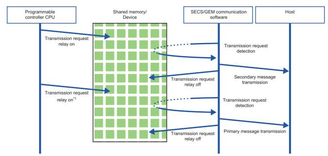
\*1 Turns ON after checking that the sending request is OFF.
