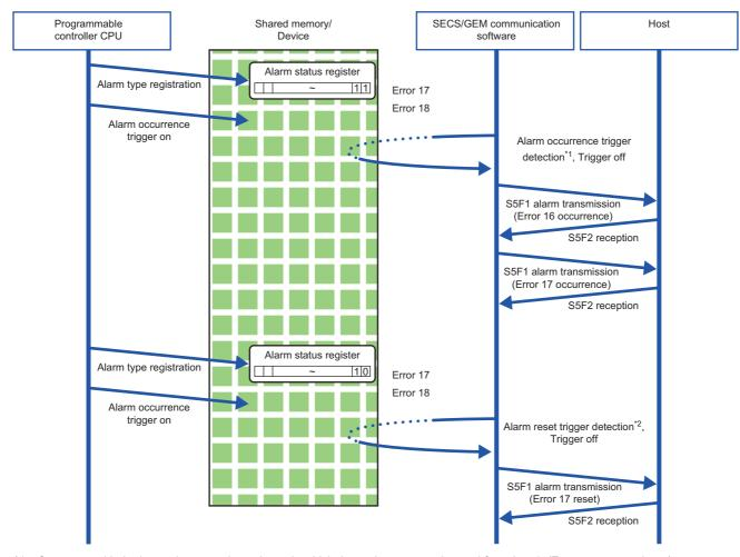
\*1 Compares with the internal state to detect items in which the register status changed from 0 to 1. (For occurrence trigger)
