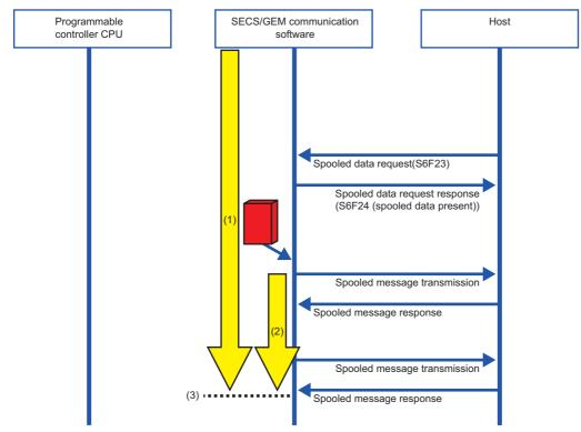
(1) The spooling relay switches ON.
