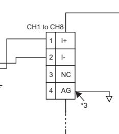
\*1 For the wire, use the shielded twisted pair cable.
