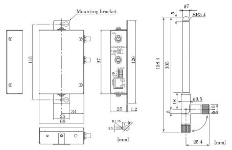
Figure 8.2. External Dimensions (when installed with mounting brackets)
