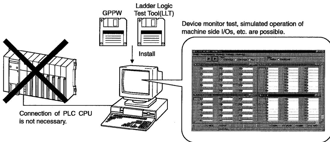
A sequence program created with GPPW can be debugged by writing it to the ladder logic test tool (LLT).
