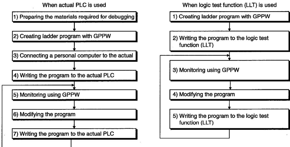
(2) Easy Debugging of FROM/TO Instructions for Special Function Modules
