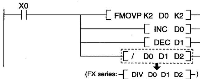
\* Some instructions differ between the A/QnA series and the FX series CPU. For details, refer to the Programming Manual of the individual CPUs.
