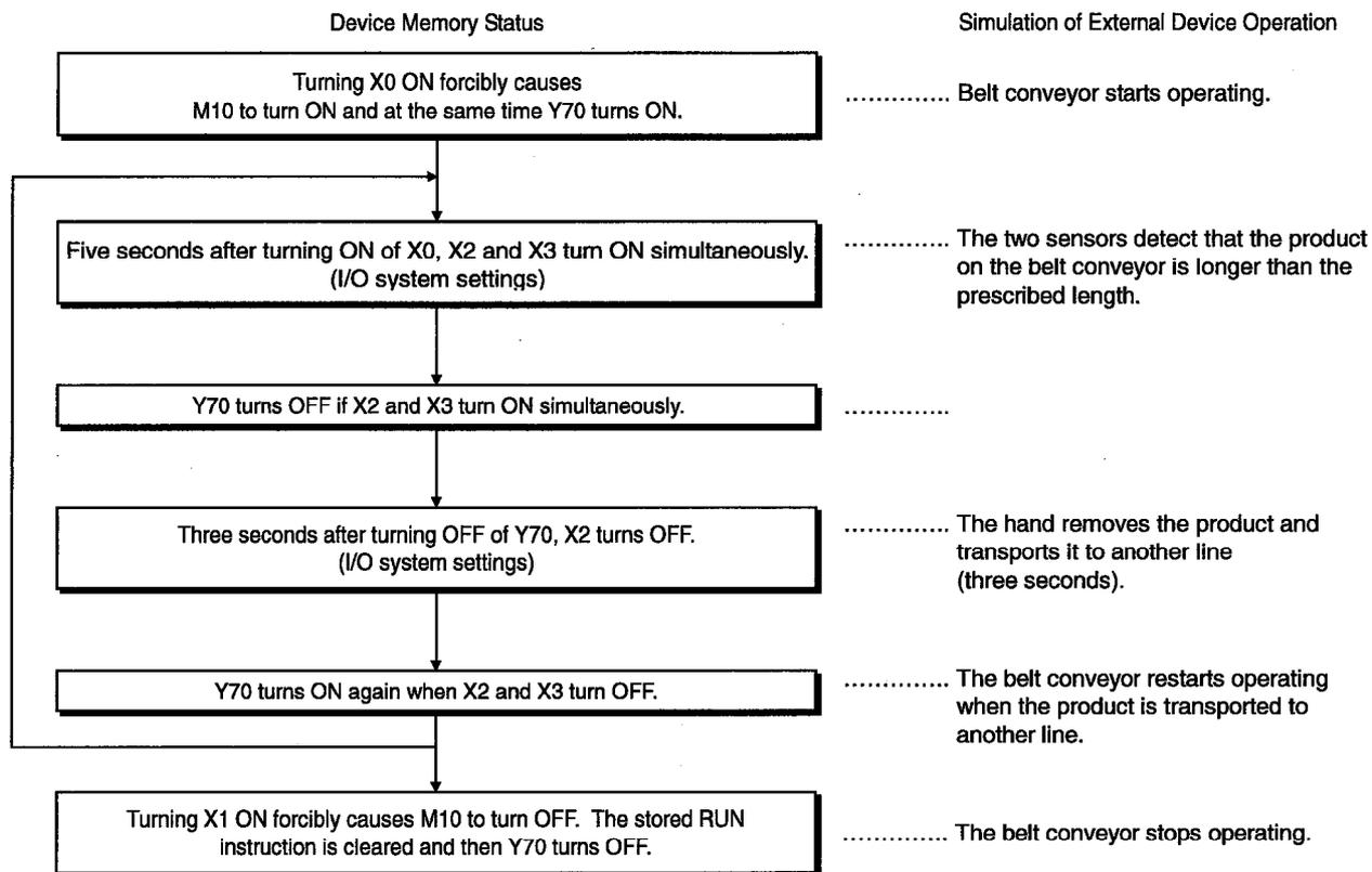
During an actual simulation, check the device memory status using the ladder logic test tool (LLT) or GPPW device batch monitor.
