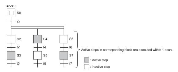
At the end of the operation output execution at each step, whether the transition condition to the next step is satisfied or not is checked.
