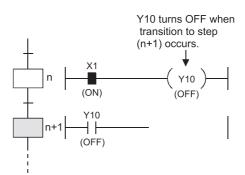
At steps not designated as coil HOLD steps, "Y10" (switched ON by OUT instruction) is automatically switched OFF when the transition condition is satisfied.
