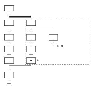
A program of a jump transition to another vertically branched ladder, a jump transition for exiting from a parallel branch, or a jump transition to a parallel branch from outside a parallel branch cannot be created.
