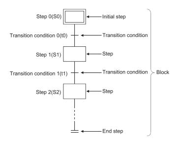
An SFC program starts at an initial step, executes a step following a transition condition in due order every time that transition condition is satisfied, and ends a series of operations at an end step.
