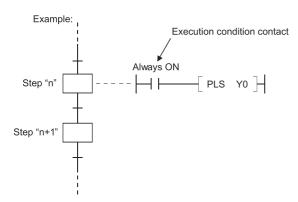
The ladder shown above is actually executed as shown below. Because the step conditions contact is ON when the step is active and OFF when the step is inactive, the PLS or  $\Box$  P instruction will be executed when the step becomes active, even though the execution condition contact is always ON.
