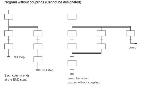
As a rule, a waiting step must be created prior to the coupling. However, in cases such as the example below where each of the parallel transition columns consist of only 1 step (program without a transition condition between the parallel transition branch and the coupling), a waiting step is not required.
