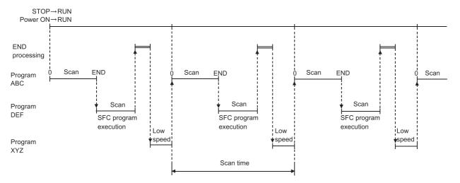
\*1 For the Universal model QCPU and LCPU, only one SFC program (one normal SFC program) can be scanned.
