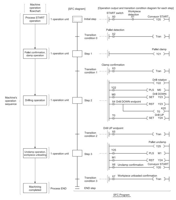
The SFC program performs a series of operations, beginning from the initial step, proceeding to execute each subsequent step as the transition conditions are satisfied, and ending with the END step.
