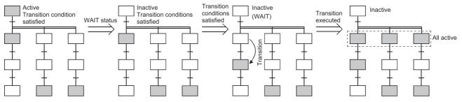
• When setting is "TRANSFER": When any one of the transition destination steps of the parallel branch is active, a transition is executed and the previous step becomes inactive.
