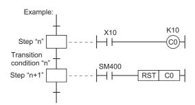
When the counter (C0) is reset at step "n+1" (or subsequent step), the present value will be cleared, and the contact will be switched OFF.
