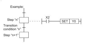
When transition condition "n" becomes satisfied at the step "n" operation output where Y0 is ON (by SET instruction), the Y0 ON status will be maintained even after the transition to step "n + 1".
