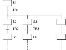
When synchronizing transitions from S2 to S5, from S3 to S6, and from S4 to S7, describe the following program at TR3 and TR4.
