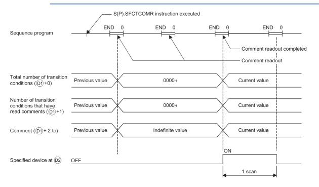
The operation when a command of S(P).SFCTCOMR instruction is in ON status at S(P).SFCTCOMR instruction execution completed is as follows.
