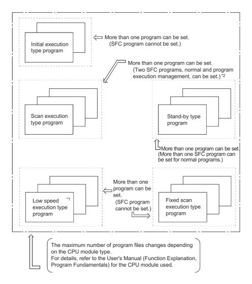
\*1 The Redundant CPU, Universal model QCPU, and LCPU cannot execute the low-speed execution type program.
