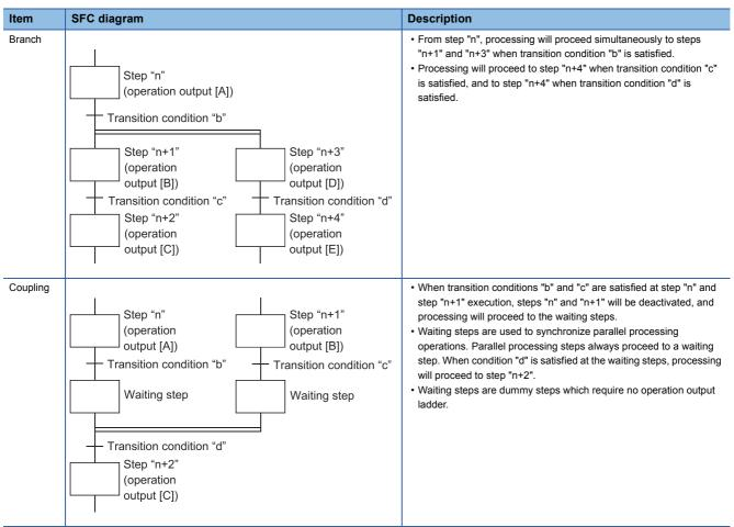
Up to 32 steps can processed simultaneously with the parallel transition format.
