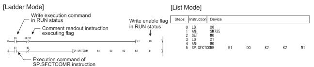
Procedure for "batch writes of SFC program in RUN status", "online change (inactive block)", or "write of comment file in RUN status"
