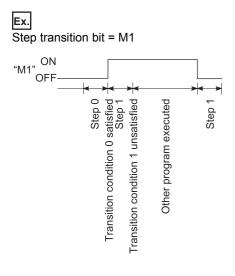
• At active parallel branch steps, the transition bit will switch ON when any of the transition conditions are satisfied.
