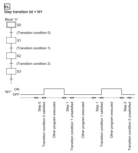
If a continuous transition is designated (continuous transition bit ON), the transition bit will remain ON during the next step's operation output after the transition condition is satisfied. It will also remain ON following the execution of multiple steps, even if the transition condition is unsatisfied. In these cases, the transition bit will switch OFF when block execution occurs at the next scan.
