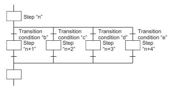
If transition conditions "c" and "d" are satisfied simultaneously, the step "n+2" operation output will be executed.
