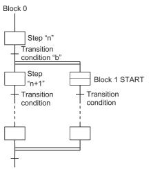
When condition "b" is satisfied at step "n" execution, processing will proceed to step "n+1" and block 1 will be started. Blocks "0" and "1" will then be processed simultaneously.
