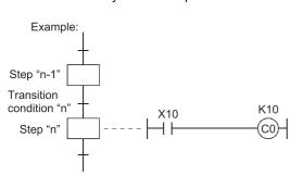
If X10 at step n is already ON while step (n-1) is active, counter C0 counts once when execution proceeds to step n after transition condition n is satisfied.
