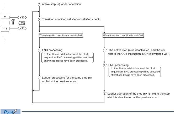
END processing is performed after all the program files set to the "scan execution type" in the program setting of the PLC parameter dialog box have been executed. Refer to the QCPU User's Manual (Function Explanation, Programming Fundamentals) for the detailed processing order of the programs other than the SFC program and their processings.
