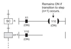
At a designated coil HOLD step, "Y10" (switched ON by OUT instruction) will remain ON even when the transition condition is satisfied.
