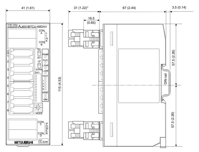
\*:This section should be 14.5mm (0.57inch) when an online connector is not installed.
