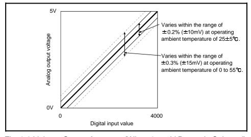
Fig. 3.2 Voltage Output Accuracy (When 0 to 5V Range Is Selected)
