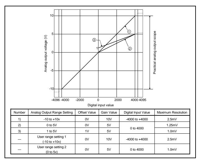
Fig. 3.1 Voltage Output Characteristic
