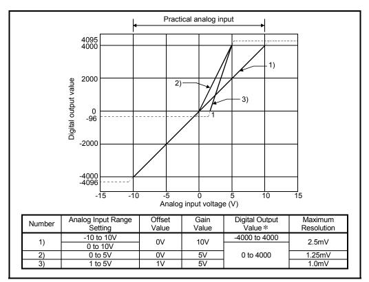
The voltage input characteristic graph is shown below.
