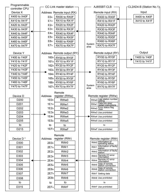
(3) Relation between programmable controller CPU, CC-Link master station, AJ65SBT-CLB and CL2AD4-B
