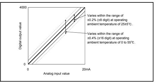
Fig. 3.4 Current Input Characteristic Accuracy
