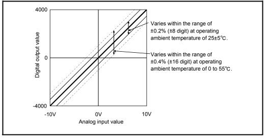
Fig. 3.3 Voltage Input Characteristic Accuracy
