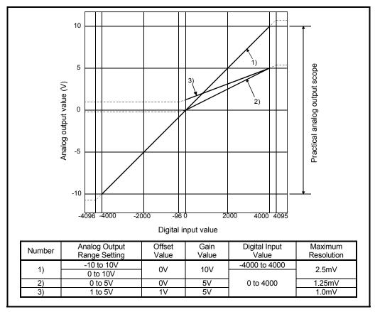
Fig. 3.1 Voltage Output Characteristic
