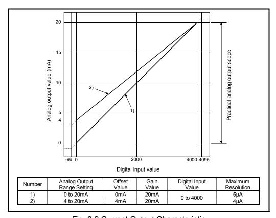
Fig. 3.2 Current Output Characteristic
