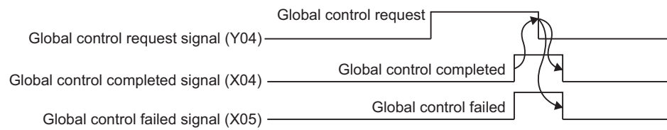
Figure 3.5 Global Control Failed Signal (X05)
